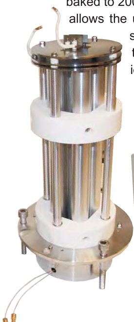
The QMF200 consists of the quadrupole (left) and power supply unit (above). In addition to a set-up page the PSU has two operational modes for scanning and filtering of the ionised clusters from the cluster source.
