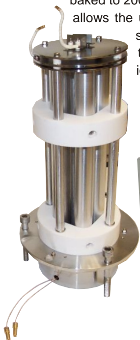
The QMF200 consists of the quadrupole (left) and power supply unit (above). In addition to a set-up page the PSU has two operational modes for scanning and filtering of the ionised clusters from the cluster source.
